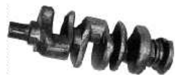
Figure 8.1: A car crankshaft is a complex three-dimensional object which is well approximated for many purposes as rotating about a fixed axis. The relative timing of the reciprocating pistons is controlled by this complex shape. “Connecting rods” are pinned to the cylinders at one end and to the short offset cylinders on the crankshaft at the other.
