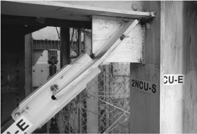
FIGURE 9.42 Ductile gusset for in plane hinging. (Courtesy of Charles Roeder, Department of Civil and Environmental Engineering, University of Washington.)
